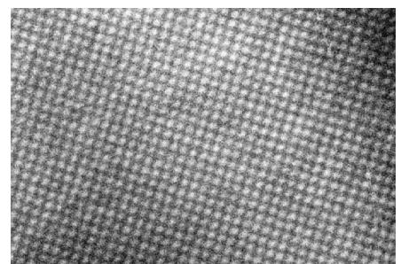
**Product No. 646****Orientated Gold Crystals**, Lattice spacing 0.204nm, 0.143nm, and 0.102nm
