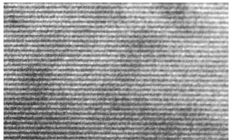
**Product No. 629-1****Copper Phthalocyanin**, Lattice plane spacing 1.03nm
